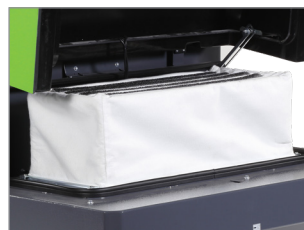
FILTER REPLACEMENT WITHOUT TOOLS
