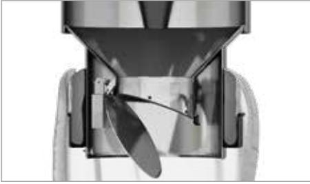
Self discharge valve with best sealing
