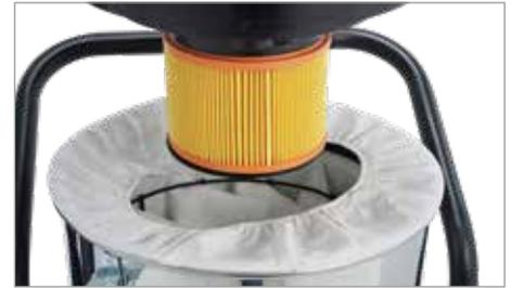
Hepa H14 cartridge and conductive prefilter
