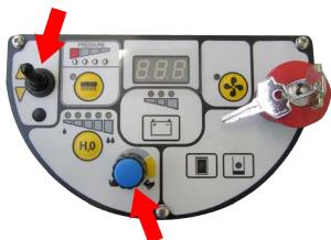
Select working pressure by turning the adjustment knob.
