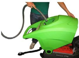
Check the suction filter is undamaged and clean.
