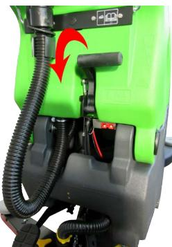
Press the brush button to enable brush rotation and turn the suction motor on.
