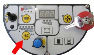
Choose the direction of movement by moving the direction selector, turn the potentiometer to set the work speed.
