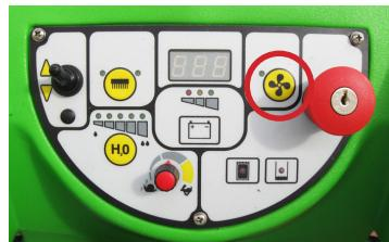
Choose the direction of movement by moving the direction selector, turn the potentiometer to set the work speed
