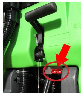
Check the detergent output filter is undamaged and clean
