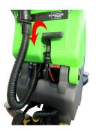
Press the brush button to enable brush rotation and turn the suction motor on.
