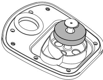
Check the squeegee is clean and the blades are not damaged.
