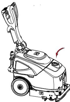
Adjust the slope of the handle by pulling the handle release lever.
