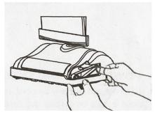
5) Rotate the brush roll several complete revolutions to ensure that no part of the belt is overhanging the end of the motor drive shaft.
