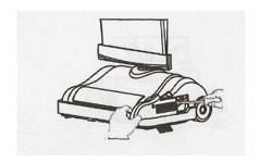
3) Remove the belt from the brush roll pulley and the motor drive shaft, clean the residue off the brush roll pulley if needed.
