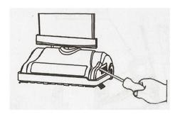
2) Slide the door forward by prying open with a screwdriver or coin.
