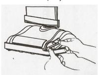
4) Loop the new belt over the motor drive shaft. Place the opposite end of the belt on the brush roll pulley.
