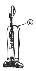
3. Press the cord into the cord clip, and ensuring the cord is fully rested in clip.
