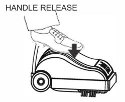
To release the handle, press on the base of the vacuum with your foot as shown at left. The handle is now free to lower for normal vacuuming.
