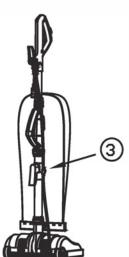
4. Connect the extension cord to the power cord male plug, and a cord connector to be used to avoid the loose connection between power cord and extension cord. (Refer to the below illustrations.)
