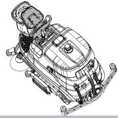
Unlock the dirty water tank from the solution tank by pulling the knob as illustrated.
