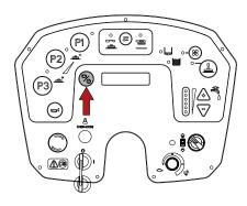
Select the type of batteries installed using the "+" or "-" button: "ACID battery" or "GEL battery".
