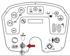
Press the brush coupling/release button, the machine will first perform a release operation, which immediately enables the coupling operation; now the machine is ready for the coupling step, which can be accomplished by pressing the brush coupling and release button a second time.
