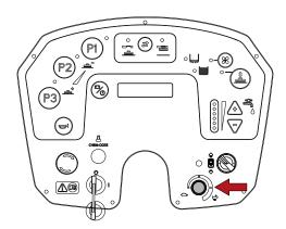
Chem Dose model, press the switch to turn on the device. To change the percentage dilution of the detergent (Chem Dose model), refer to the section "Selecting the percentage dilution of the detergent (Chem Dose model)".
