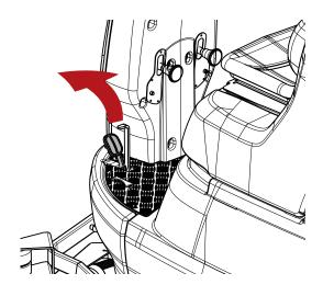
To release the parking brake, press the lever next to the pedal.
