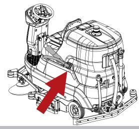
or use the hose with ACQUA-STOP fill system (model with ACQUA-STOP). Once the quick coupling hose is connected to the machine, this device allows the tank to be filled without the presence of the operator. Dispensing will be stopped automatically when the tank is filled.
