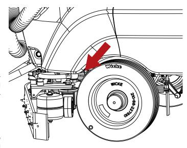
On machines equipped with Chem Dose (Chem Dose model), make certain that the detergent flow valve is open.
