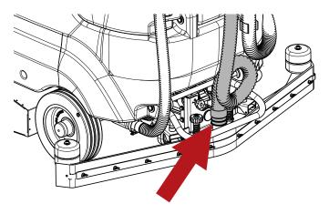
Tighten the two knobs.
