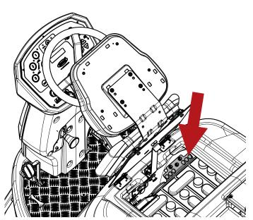
The machine is equipped with resettable fuses also known as thermal fuses. These are resettable devices serving to protect the electrical circuits, which shut off the flow of current in the event of an overload. Once the thermal fuse has been tripped, allow time for it to cool, then press the reset button to restore normal operation.
