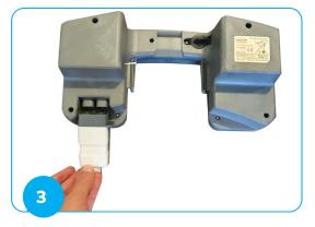
3. Please connect the 2 pin connector to the battery. It will only fit correctly in one direction. (C in figure 4)
