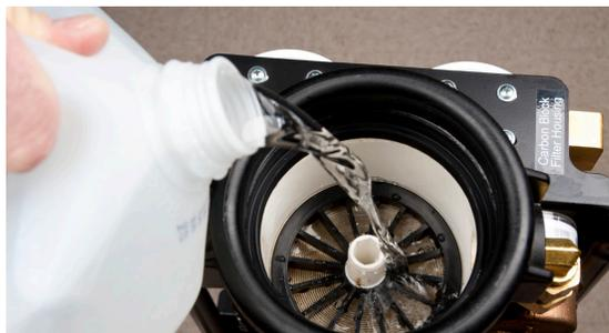
Slowly pour solution into the top of the open RO pressure vessel(s). Reinstall green hose to the inlet when the solution starts coming out.
