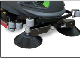
PRE-SWEEP SYSTEM ON CYLINDRICAL MODEL
