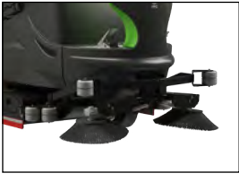
PRE-SWEEP SYSTEM ON CYLINDRICAL MODEL
