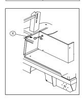
If the machine is in the DP version, it must be filled with lead-free petrol or diesel, depending on the engine. A label indicating the kind of fuel to use is in any case applied near the fuel cap. Check the level of oil in the engine
