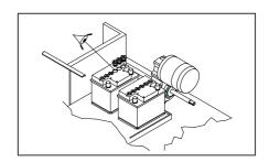
2 If the batteries are supplied without liquid (i.e. dry), they must be filled with sulphuric acid (density from 1.27 to 1.29 kg at 25℃), according to the instructions given in the next paragraph and in the battery handbook:
