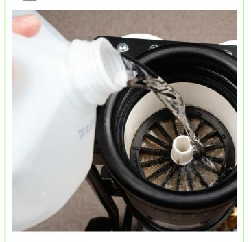
Slowly pour solution into the top of the open RO pressure vessel(s). Close drain/flush valve when solution starts coming out, filling pressure vessel(s) to the top.
