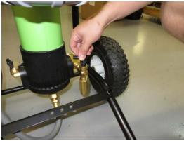
4. Remove black plastic elbow from bypass valve. The elbow can be thrown away.
