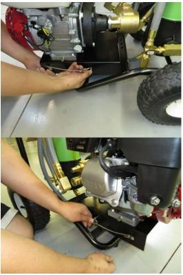
10. Attach motor to cart by inserting pins into the mounting bracket.
