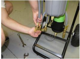
7. Connect hose from carbon block filter housing to brass connector block. Use Teflon tape. Wrench 7/8"
