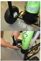
8. Remove flow restrictor. Replace with provided new one. Use Teflon tape. Wrench 1 1/16"
