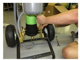
6. Install short hose from brass connectors into bypass valve. (Where black plastic elbow was removed from step 4) Use Teflon tape on threads. Wrench 11/16"
