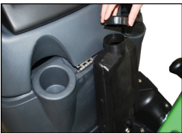
SEPARATE DETERGENT DOSING SYSTEM
