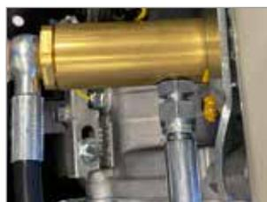
ACOPLAMIENTO FLEXIBLE ENTRE BOMBA Y MOTOR
