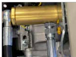
ACOPLAMIENTO FLEXIBLE ENTRE BOMBA Y MOTOR
