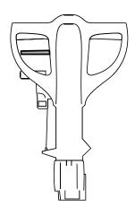
Press the brush button to activate suction and water delivery.
