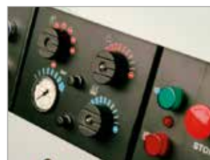
CONTROL PANEL PROVIDED WITH EMERGENCY SHUTDOWN
