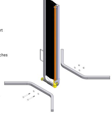
Step 2. Attach Foot Control Lever to ball valve.
